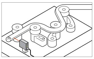
Balluff's BOD 26K analog distance sensors are highly accurate, as low as 20 micron resolution, Class II laser measurement devices. With operating ranges between 45 and 85 mm, they are perfect for use where high precision, tight tolerance and longer distance measurement is required. Bend angles, weld seams, metal-formed feature detection and validation, plus other quality inspection steps can be reliably accomplished with the BOD 26K.
